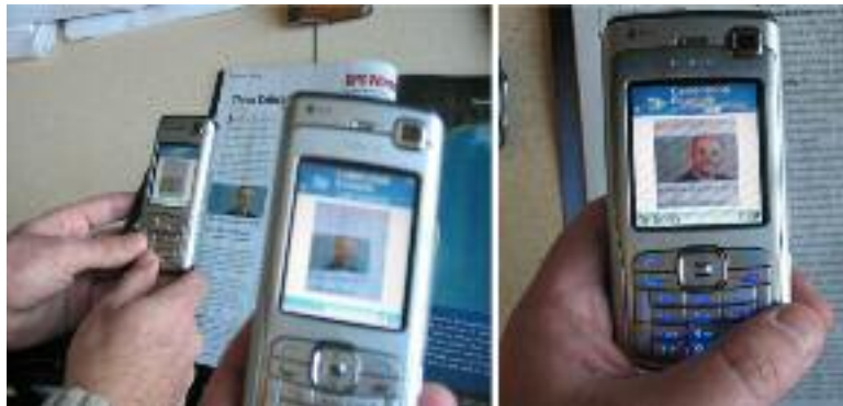
Figure 7. Real-time face detection on Nokia phone N70 with multi-resolution encoded images transferred over the Bluetooth. Bandwidth reduction from 220K (bmp) or 62 K (jpeg) to 2K.
