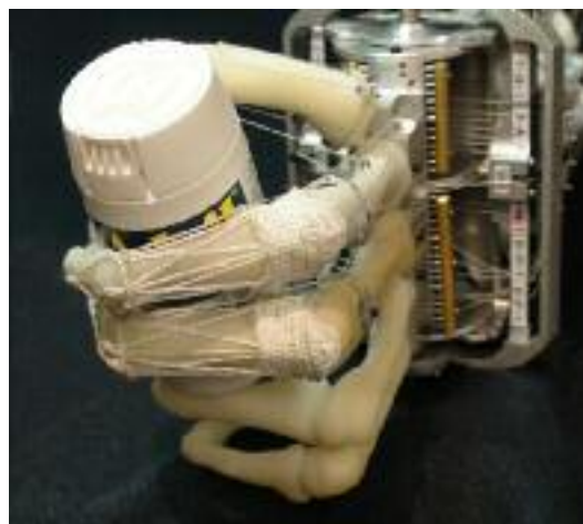
Figure 3. ACT Hand showing anatomical bone segments with muscle-motors acting via 'tendons' with realistic insertions and redundancy.
