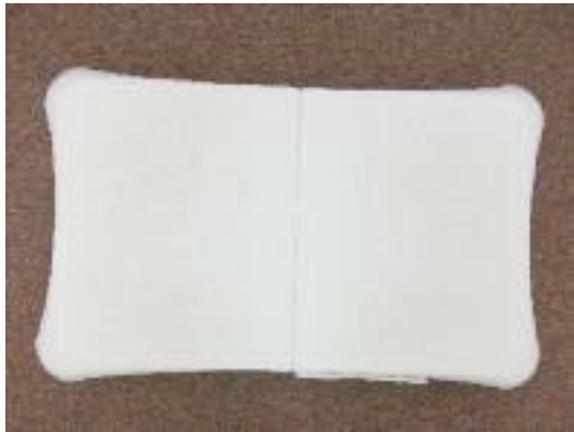
Figure 1. The Wii Fit Balance Board™ weighs 10 pounds, with the dimensions of 20.5 x 3.2 x 13.4 inches.
