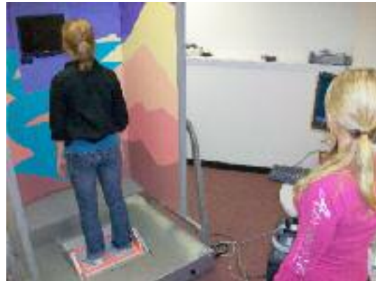
Figure 5. Subject performing a trial of the Weight Bearing Squat on the EquiTest® without her feet aligned. She is standing in a natural stance to simulate the stance that is used on the Wii Fit Balance Board™.
