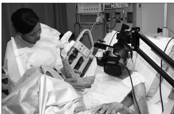
FIGURE 1A AND 1B. U.S. Army soldier receiving immersive Virtual Reality to reduce his pain during severe burn wound care, using our unique articulated arm mounted VR goggles designed by Hoffman and Magula, that hold the displays near the patient's eyes. Photos and copyrights Hunter Hoffman, UW.
