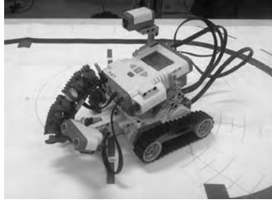
Figure 1. Robot which is able to move and shoot balls if there an object along its route.
