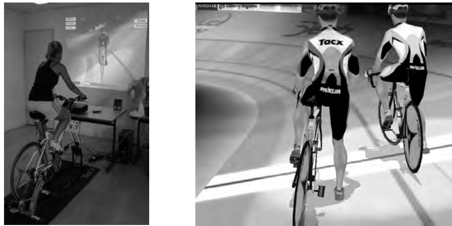
Figure 1. Left: The participant was pedaling on a standard stationary bike connected to a computer running the Tacx ® VR software. The computer was connected, via USB, to a pad, fixed to the real wheel of the bike. This pad had two functions. First, after calibration, it measured the bicycle's rear wheel rotation, hence, directly controlling the virtual cyclist's displacement speed in the virtual world. Secondly, it opposed, a variable resistance to the participant's pedaling effort through an electromagnetic brake. In our case, using an indoor circuit, the resistance level was kept constant. Right: Representation of the participant's avatar (center of the picture). In one experimental condition (see below), a second avatar was present in the VE (right of picture), acting as a virtual coach (or pacer).
