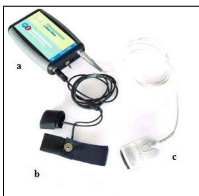
Figure 3. GSR/HR Sensor Module: a) the control box; b) the Skin Conductance Response sensors; c) the Blood Volume Pulse sensor (developed by Aurelia)
