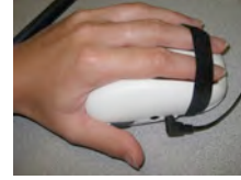
Fig. 2.a GSR2 skin conductance device
