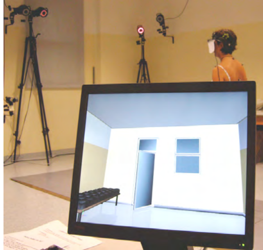
Figure 2. The image on the screen is the same of that one displayed on HMD and represents the virtual laboratory seen from the avatar perspective, while subject is walking.
