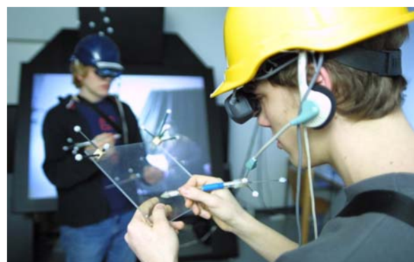
Figure 2. Two students collaborate in our standard lab setup, wearing an HMD, holding a wireless pen and panel. All devices are optically tracked.
