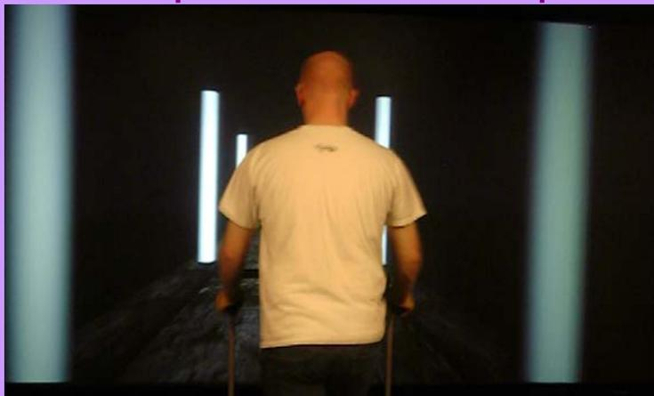
Non-motorised treadmill in front of a 5m wide stereoscopic display
