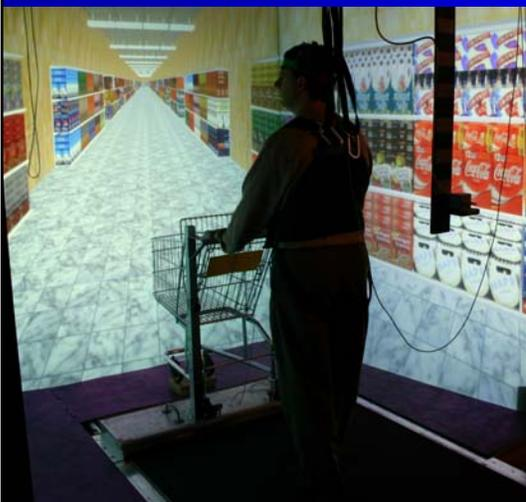
Subjects walked through a virtual grocery store while pushing on a grocery cart instrumented with force transducers.
